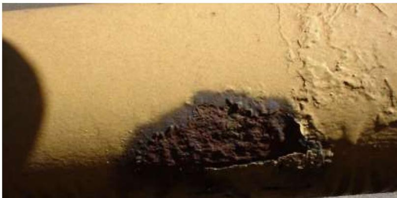
**LA PROTECTION PASSIVE** = PROTECTION PAR REVETEMENT
